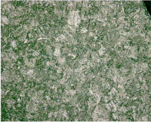
Photo 48. Structure of the MP-3-III comparative cutter knife steel. Magnification 200 x.
