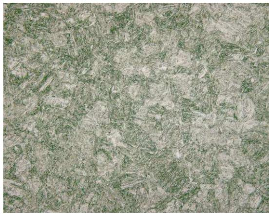
Photo 47. Structure of the MP-3-II comparative cutter knife steel. Magnification 200 x.
