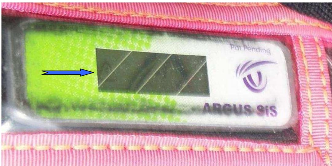
Photo 8. LCD damage. Blue arrow points a flashing sign.
