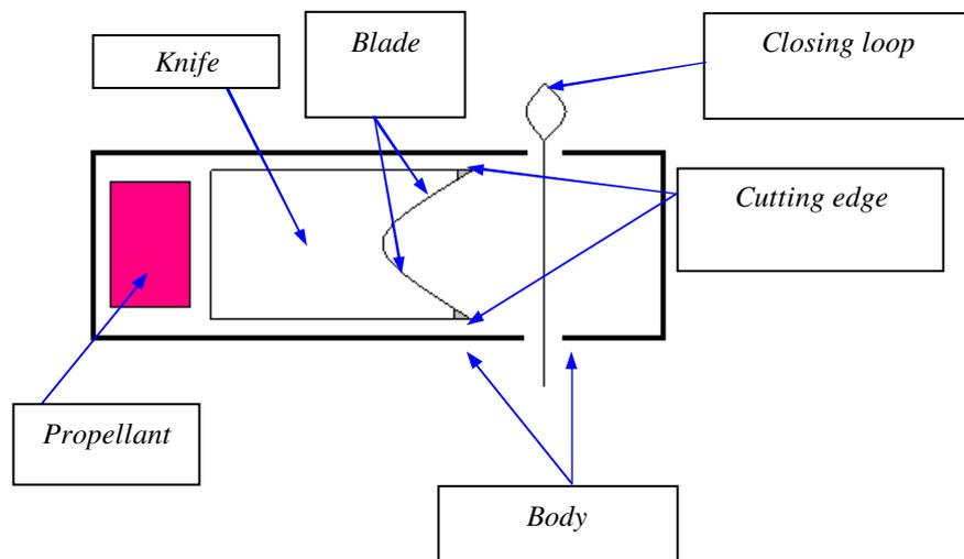
Fig.1. Diagram of the "Argus" AAD cutter.
