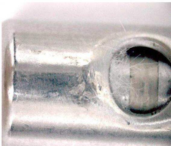
*Photo 26. Visible fibers of the closing loop protruding from the hole of the cutter secured on the scene.*
