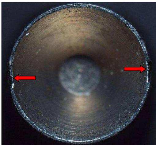
*Photo 40. Experimental cutter MP-5. Knife view from the blade side. Red arrows indicate damage to the cutting edge of the knife blade.*
