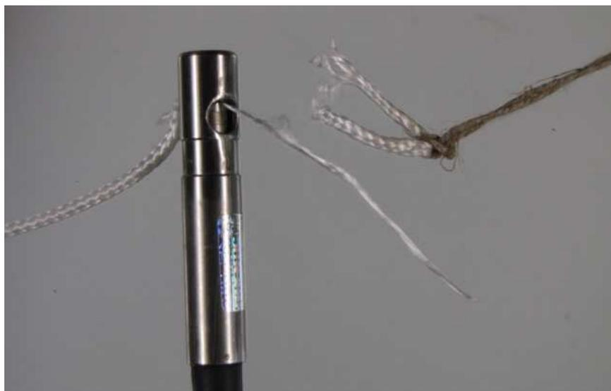
*Photo 39. View of the MP-5 cutter and two parts of the loop after experimental activation of the cutter.*
