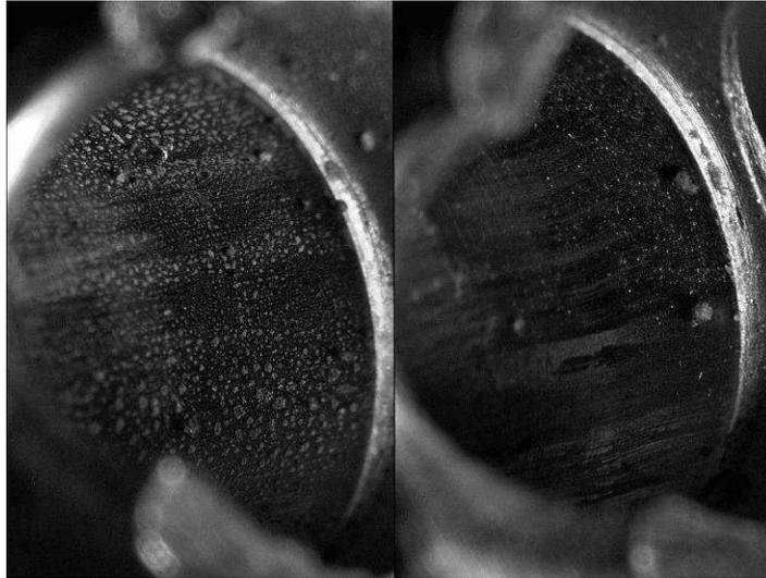
*Photo 42. Inner surfaces of the body of the cutter secured at the accident site and the comparative cutter.*
