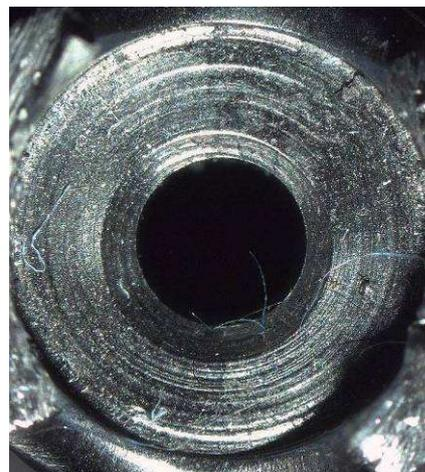
*Photo 41. Body bottom. Lack of circular indentation corresponding to the knife diameter.*
