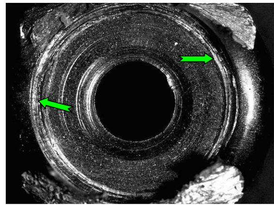
Photo 31. Body bottom. Green arrows indicate circular indentation corresponding to the knife diameter.
