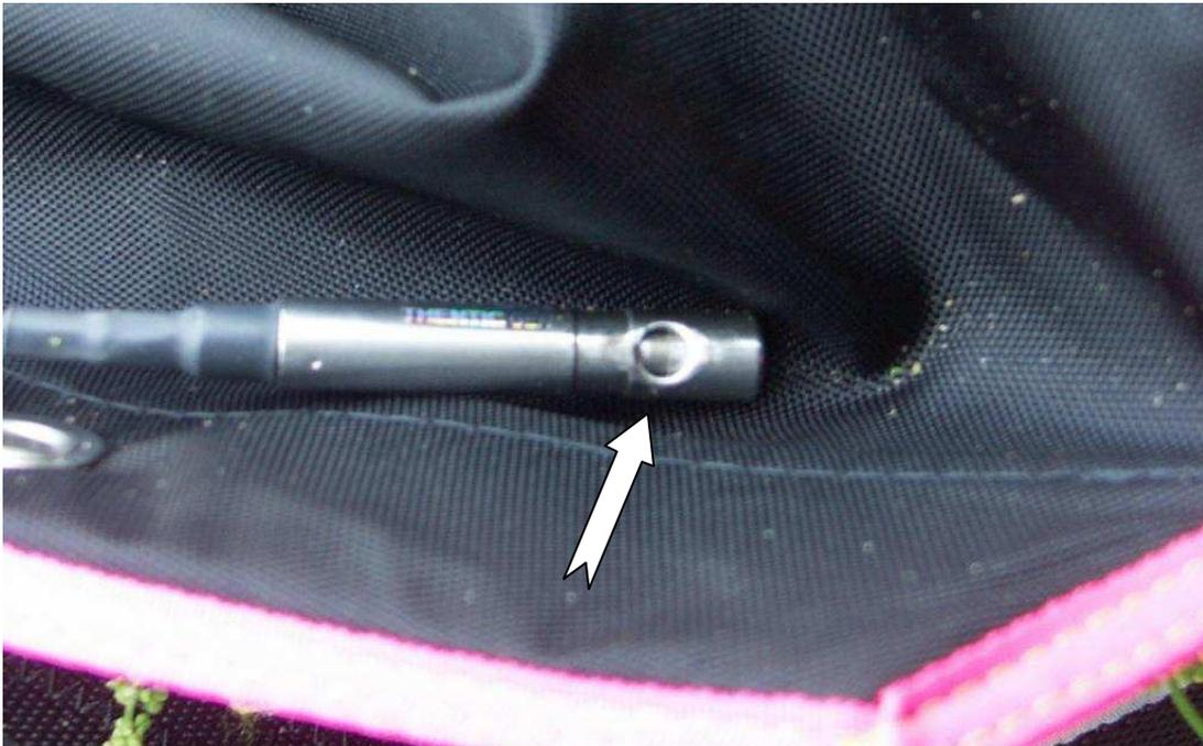
*Photo 3. AAD cutter. White arrow points a hole in the cutter body closed by knife.*
