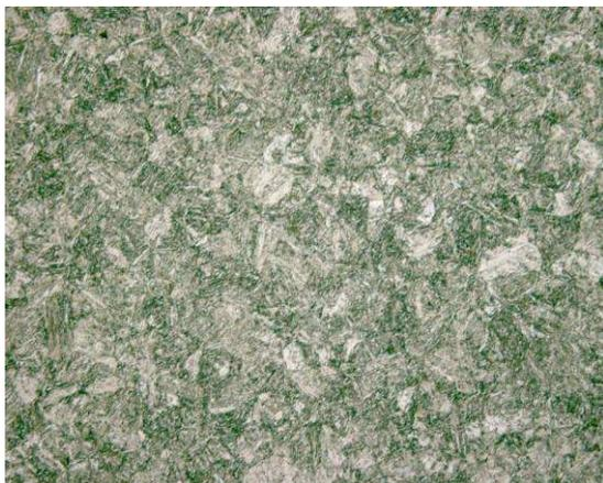
Photo 46. Structure of the MP-3-I comparative cutter knife steel. Magnification 200 x.
