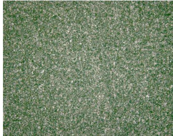
Photo 45. Structure of the MP-2 cutter knife steel. Magnification 200 x.
