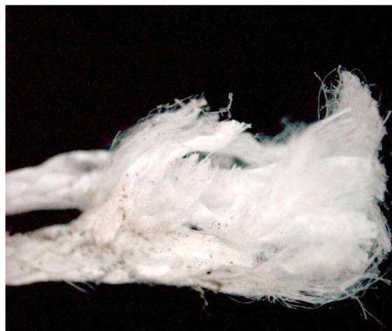
*Photo 27. Closing loop secured on the scene (partially cut and partially torn).*
