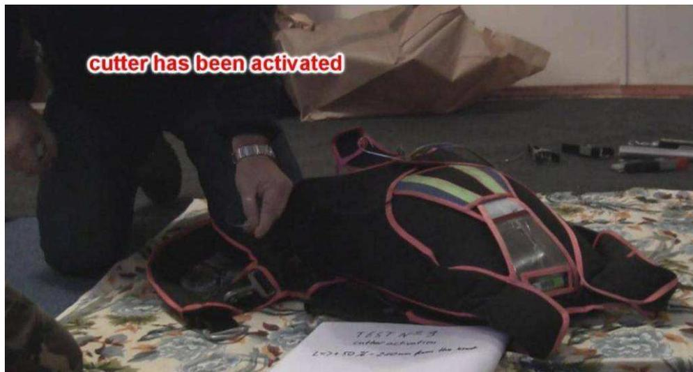
*Photo 10. Parachute just after cutter activation. The reserve canopy container was still closed.*
