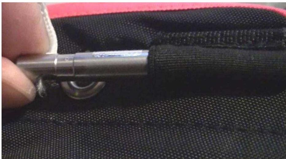
*Photo 17. Visible fibers of the upper part of the closing loop, protruding from the zipper.*
