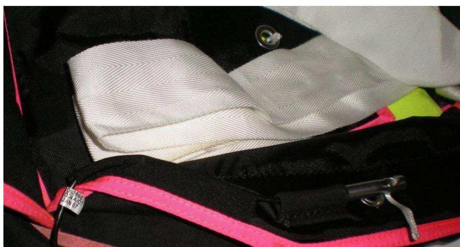
*Photo 19. View of the reserve canopy container after the pilot chute was moved aside.*
