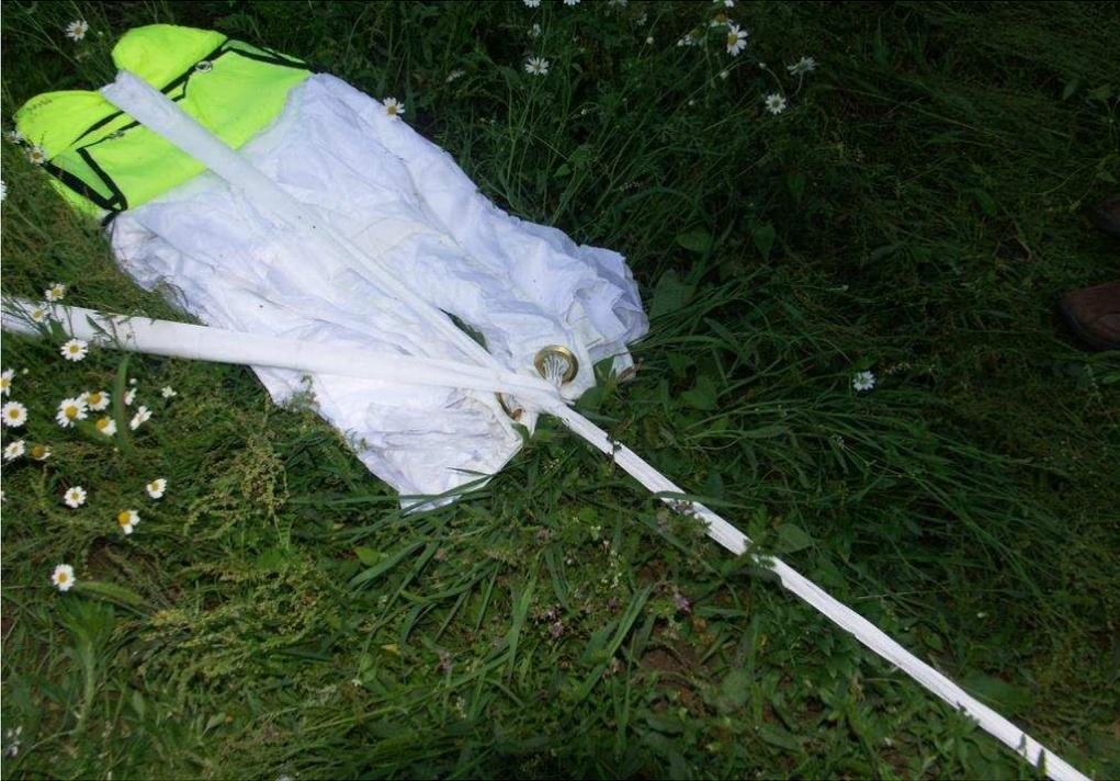
*Photo 2. Reserve canopy partially pulled out of a bag and lines wrapped by bridle.*
