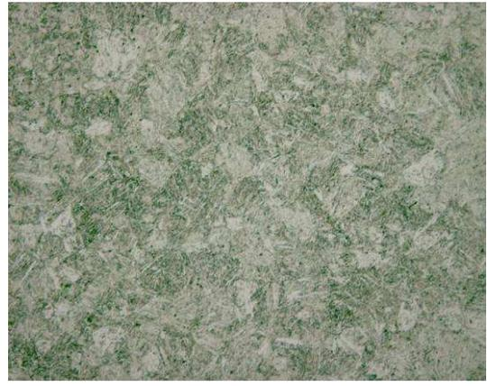
Photo 49. Structure of the MP-5 comparative cutter knife steel. Magnification 200 x.
