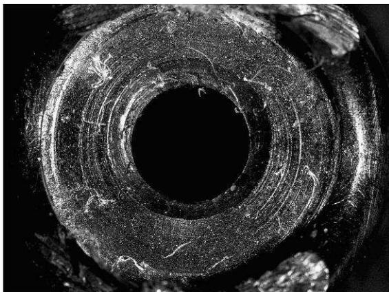
Photo 30. Body bottom. Lack of indentation corresponding to the knife diameter.
