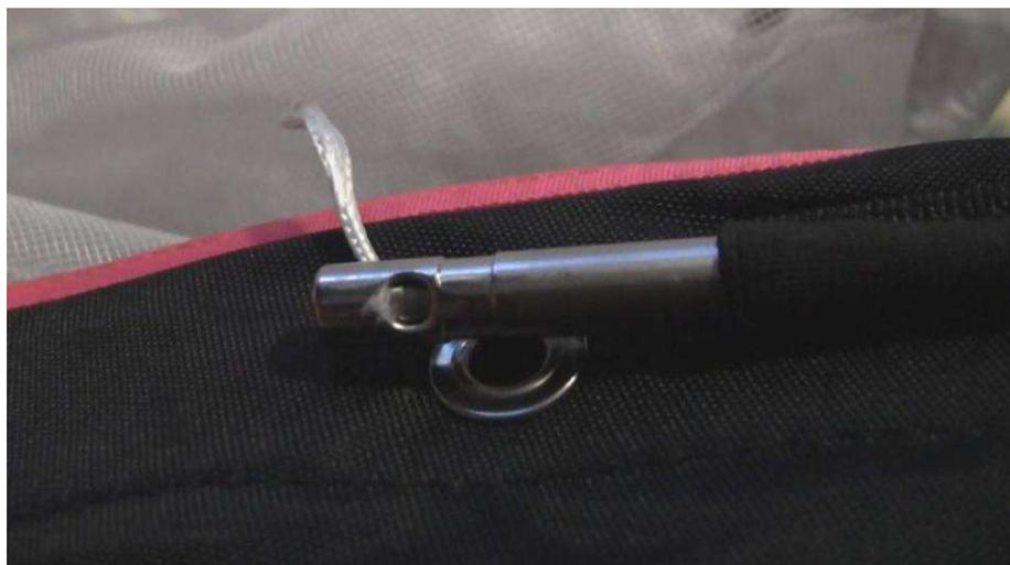
*Photo 16. Upper part of of the closing loop, manually broken. The photo shows, that the cutter cut only a part of the fibers.*
