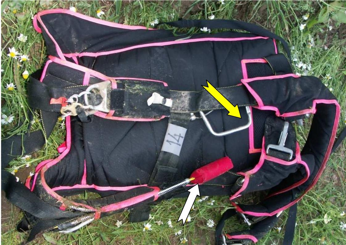
Photo 7. Back part of the harness/container. Visible main canopy cut away handle (white arrow) and reserve canopy opening handle (yellow arrow) - both not pulled out.
