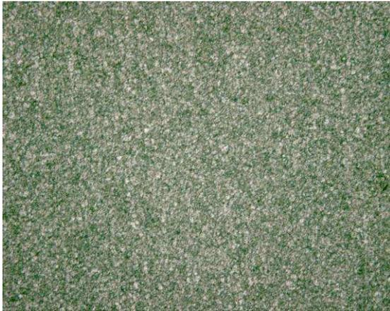
Photo 44. Structure of the MP-1 comparative cutter knife steel. Magnification 200 x.
