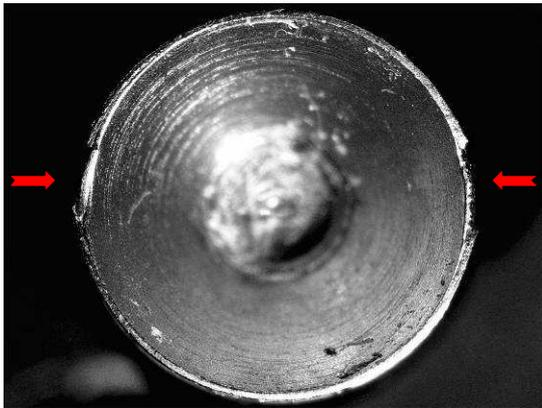
Photo 28. Cutter secured on the scene. Knife view from the blade side. Red arrows indicate damage to the cutting edge of the knife blade.
