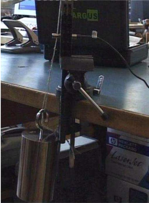
*Photo 33. View of MP-5 cutter and the loop prior to propellant activation.*
