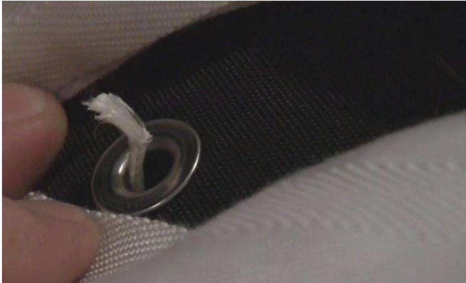
*Photo 20. Close-up of the lower part of the closing loop. Frayed fibers endings are clearly visible.*
