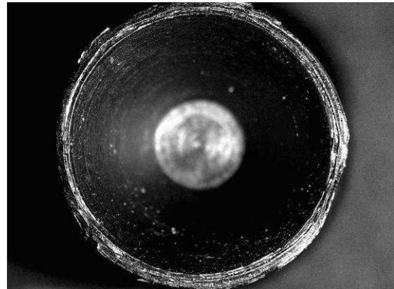
Photo 29. Cutter used by the manufacturer for demonstration. Knife view from the blade side. Material from the body bottom visible on the cutting edge of the knife blade.
