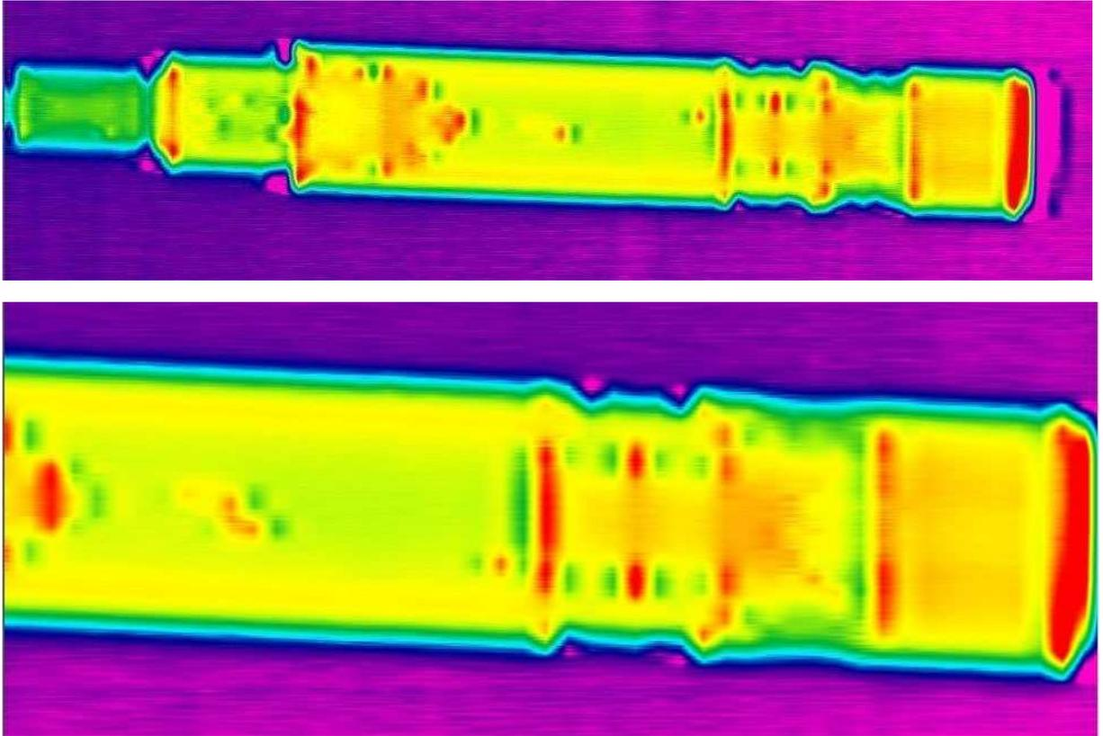
Photos 22-25. X-rays of the cutter secured at the accident site.
