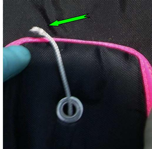
*Photo 5. Lower part of the closing loop. Green arrow points irregular, frayed ending of the separated closing loop.*
