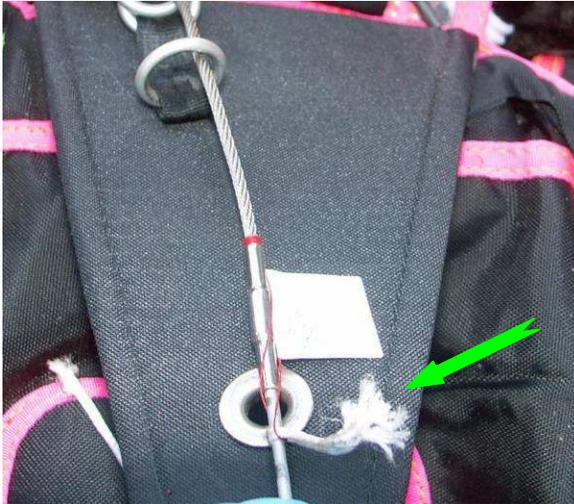
*Photo 4. Pin of the reserve canopy opening handle and upper part of the closing loop. Green arrow points frayed ending of the separated closing loop.*
