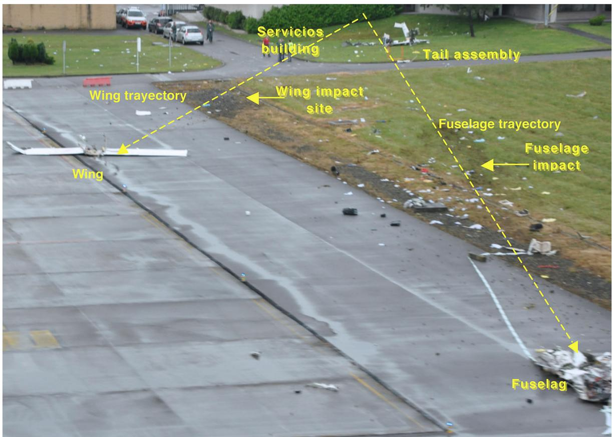
Figure 7. Photograph of wreckage taken from the runway
