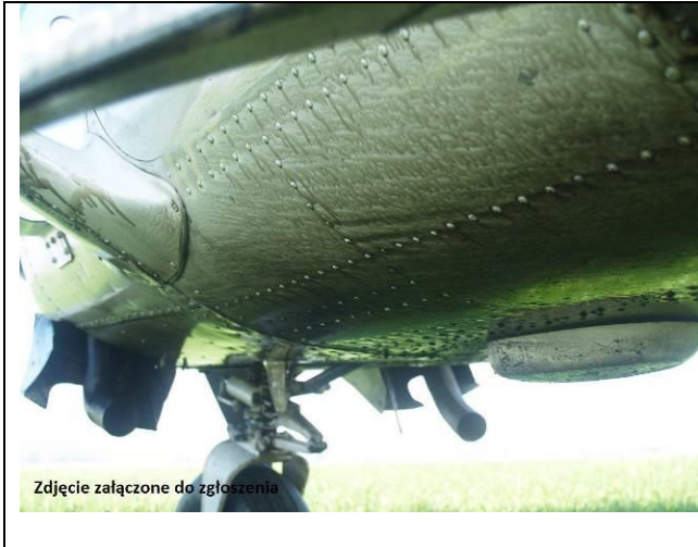
Figure 1. Lower surface of the fuselage covered with the leaking oil.
