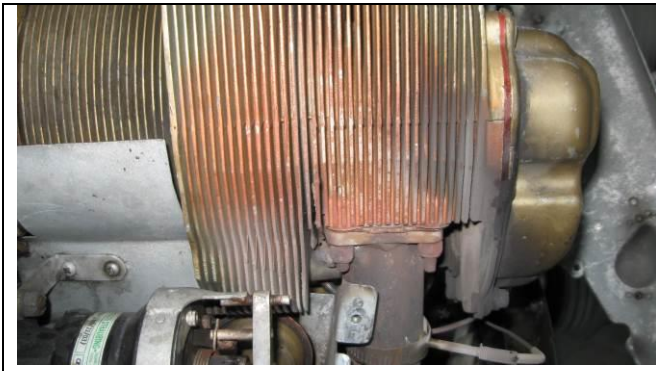
** Figure 5. Cylinder No. 6. Visible blowthrough from the cracked exhaust manifold.
