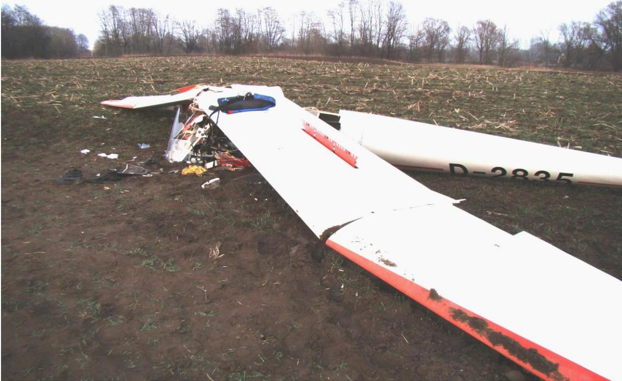
**Figure 2. The glider after the accident. Visible the front part of the fuselage - completely destroyed.**
