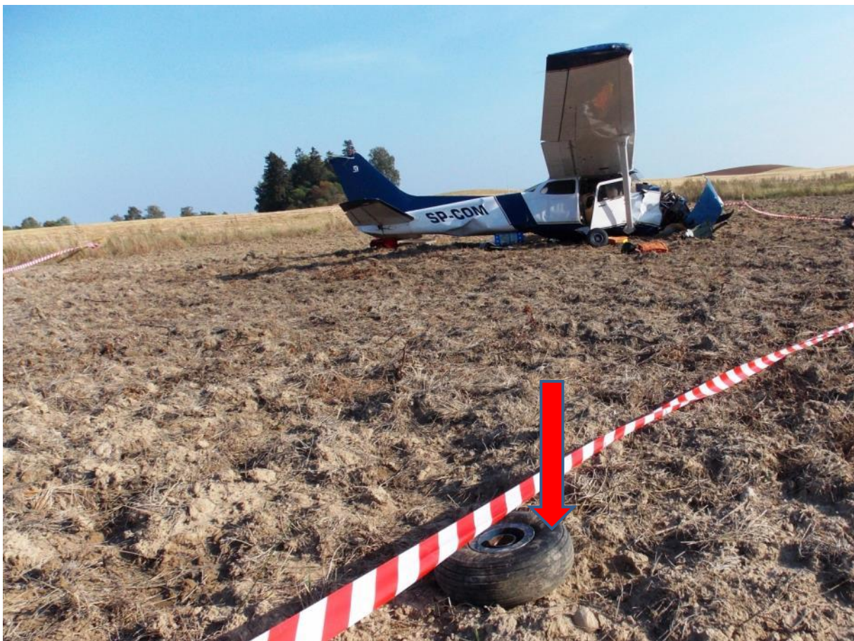
Fig. 3. The plane after stopping, red arrow shows the separated nose wheel [source: PKBWL]
