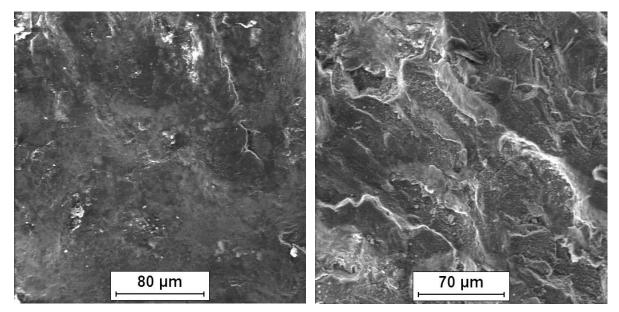
Fig. 22. Fatigue crack from the upper area marked in fig. 20. Visible light fatigue striations [source: Silesian University of Technology]
