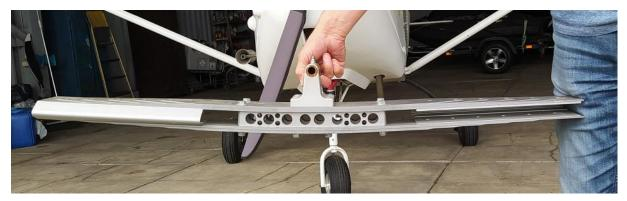
Fig. 31. Example of a gyroplane rotor blade connector with dihedral reducing the bending moment acting on working blades [source: PKBWL]
