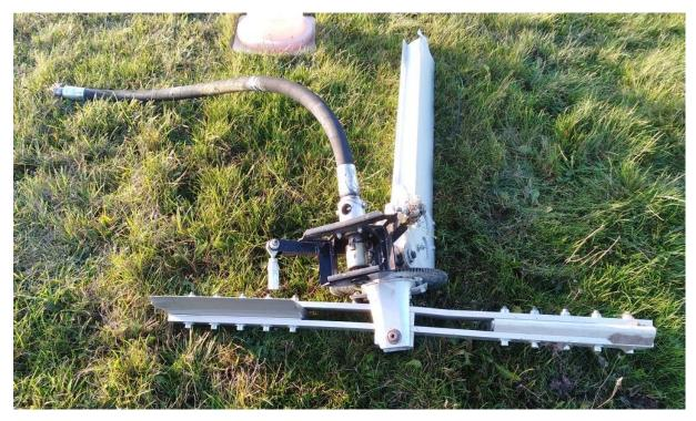
Fig. 9. The main rotor mast separated from the wreck [source: PKBWL]
