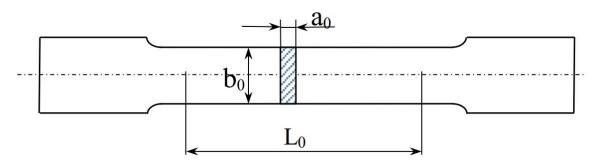
Fig. 25. A flat sample with the heads for static tensile test [source: Silesian University of Technology]
