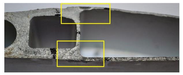
Fig. 19. Sampling areas for examination with the scanning electron microscope [source: Silesian University of Technology]
