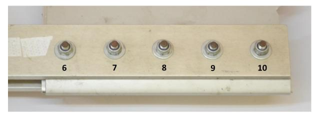
Fig. 18. Markings of the bolts of blade that broke due to destruction of the first blade [source: Silesian University of Technology]
