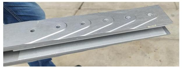
Fig. 28. Example of a gyroplane rotor blade connector with gradual change of its stiffness by changing its thickness [source: PKBWL]
