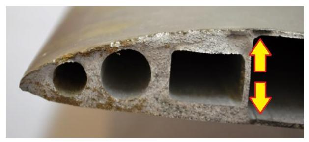
Fig. 15. The surface of the blade fracture. Places selected for examination with the scanning electron microscope [source: Silesian University of Technology]
