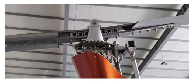
Fig. 32. Example of a gyroplane rotor blade connector with dihedral reducing the bending moment acting on working blades [source: PKBWL]
