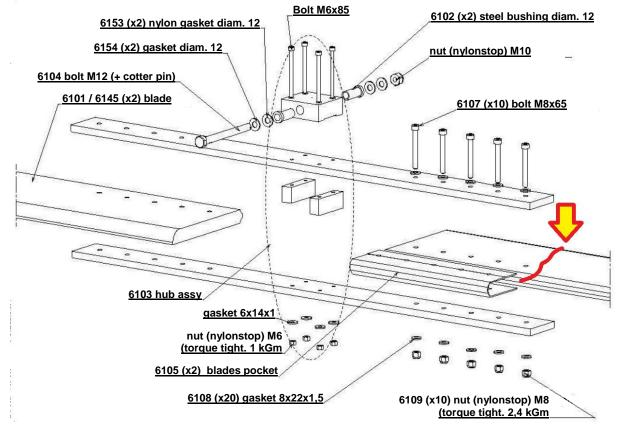
Fig. 27. ZEN1 gyroplane rotor hub assembly diagram. The arrow marks the place of the blade fracture. [source: ZEN1 gyroplane maintenance manual]
