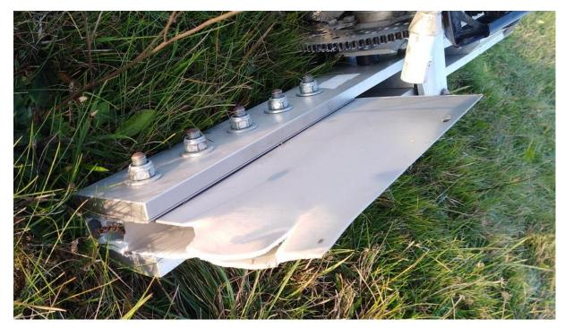
Fig. 12. View of the gyroplane rotor blades connector [source: PKBWL]
