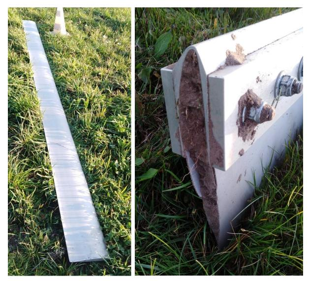
Fig. 5. Left: main rotor blade separated inflight; Right: blade connector on the main rotor hub - place where the first blade was separated [source: PKBWL]
