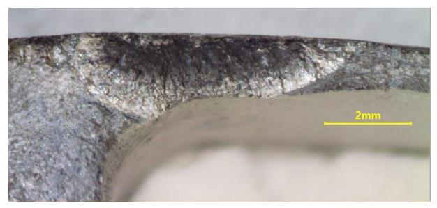
Fig. 20. Detail from fig. 19 - upper area. Visible place of the fatigue crack [source: Silesian University of Technology]
