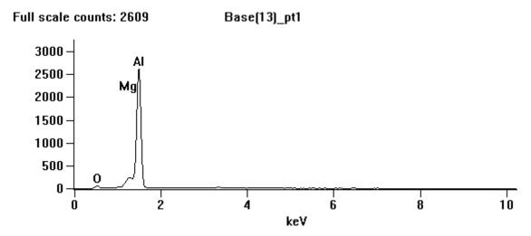
Fig. 24. X-ray microanalysis of the rotor blade chemical composition [source: Silesian University of Technology]
