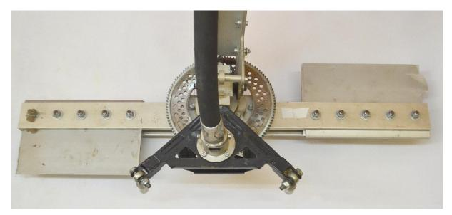
Fig. 16. The main rotor mast of the gyroplane subjected to the research - the lower part of the hub view. On the left, a fragment of the blade which was separated as first; on the right, a fragment of the other blade, destroyed due to the accident [source: Silesian University of Technology]
