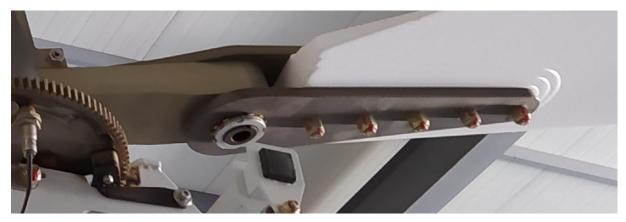
Fig. 30. Example of a gyroplane rotor blade connector with gradual change of its stiffness by changing its width [source: PKBWL]
