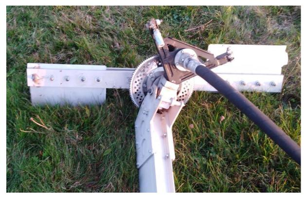
Fig. 10. The main rotor mast separated from the wreck - lower part of the hub. On the left, a fragment of the blade which was separated as first; on the right, a fragment of the other blade, damaged as a result of the accident [source: PKBWL]
