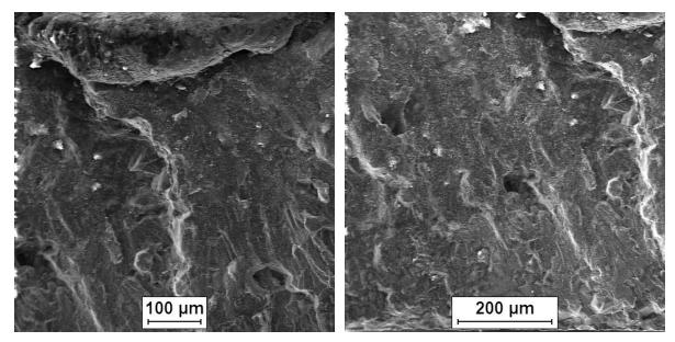
Fig. 23. Fatigue crack from the lower area marked in fig. 20. Visible light fatigue striations [source: Silesian University of Technology]
