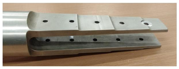
Fig. 29. Example of a gyroplane rotor blade connector with gradual change of its stiffness by changing its thickness [source: PKBWL]
