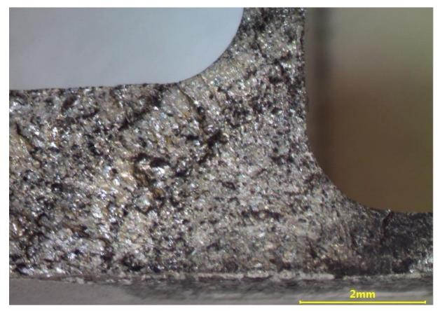
Fig. 21. Detail from fig. 19 - lower area. Visible place of the fatigue crack [source: Silesian University of Technology]
