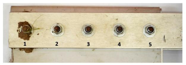
Fig. 17. Markings of the bolts of the blade detached as first [source: Silesian University of Technology]
