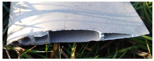
Fig. 4. Fracture of the main rotor blade, which was first detached from the connector [source: PKBWL]
