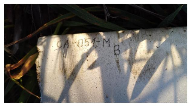
Fig. 6. Marking revealed on the separated blade found on the accident site [source: PKBWL]
