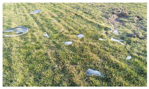
Fig. 8. The cluster wreckage that fell to the ground after the inflight disintegration of the gyroplane [source: PKBWL]
