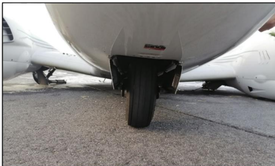
Fig.3. Nose landing gear damaged
