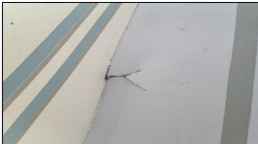
Fig.6. Damaged airframe in the wing connection area.
