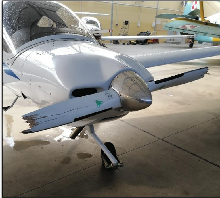
Fig. 1. Damaged propeller and nose landing gear [source: PKBWL]
