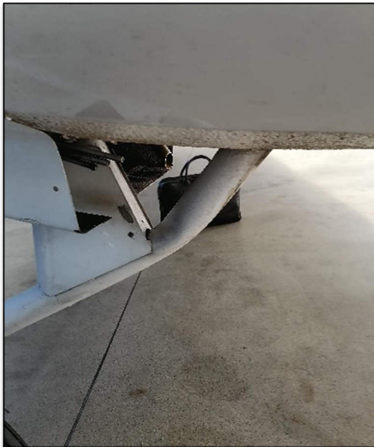
Fig. 2. Damaged nose landing gear [source: PKBWL]
