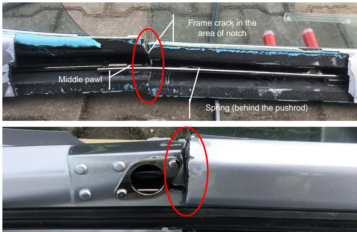
Fig. 8 Cracked canopy frame in the area of middle pawl location. A notch is present on the edge of fitting slot reinforcement [source: SCAA]
