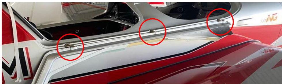
Fig. 4 Location of canopy hinges on the aircraft starboard [źródło: PKBWL]
