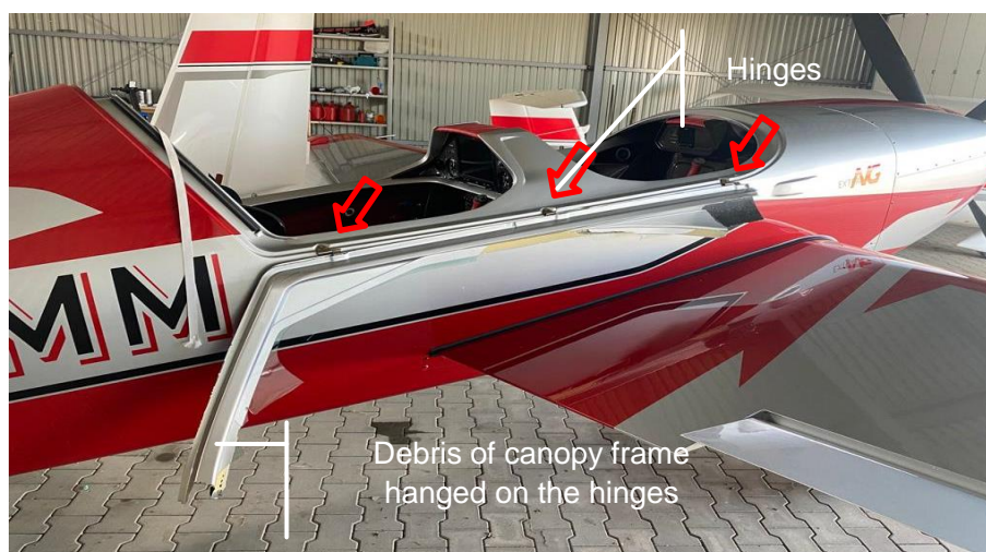
Fig. 2 Cockpit of the aircraft and a part of the broken canopy frame [source: SCAA]
