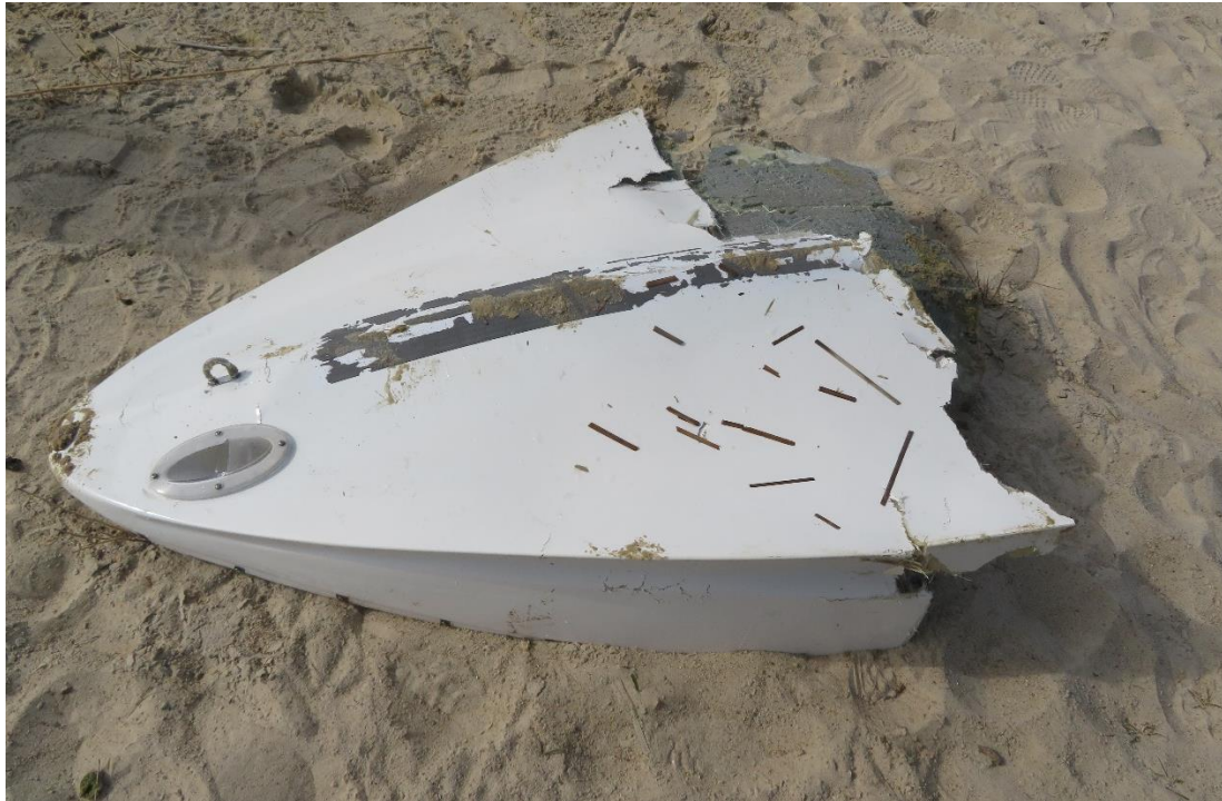
Fig.3 Detached lower part of the fuselage [source: PKBWL]
