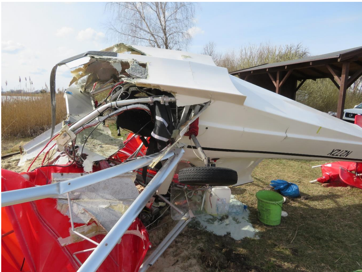
Fig.2 Nose part of the fuselage in an inverted position after the occurrence [source: PKBWL]
