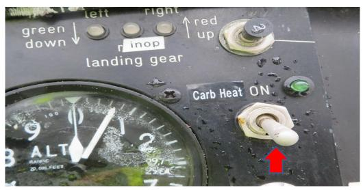
Fig. 9. Carburetor heating switch in off position [source: PKBWL]
