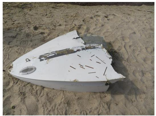
Fig. 4. View of the detached lower part of the fuselage [source: PKBWL]
