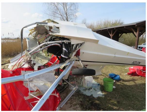
Fig. 3. View of the damaged front part of the fuselage in inverted position [source: PKBWL]
