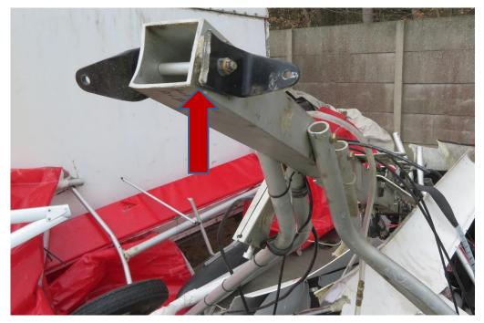
• Broken hinge of the front spar of the left wing (Fig. 8).
