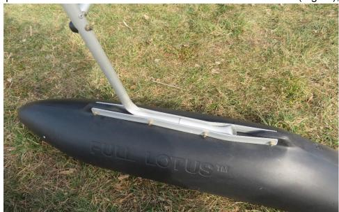
separated left float from the airframe after collision with water (Fig. 7.);
