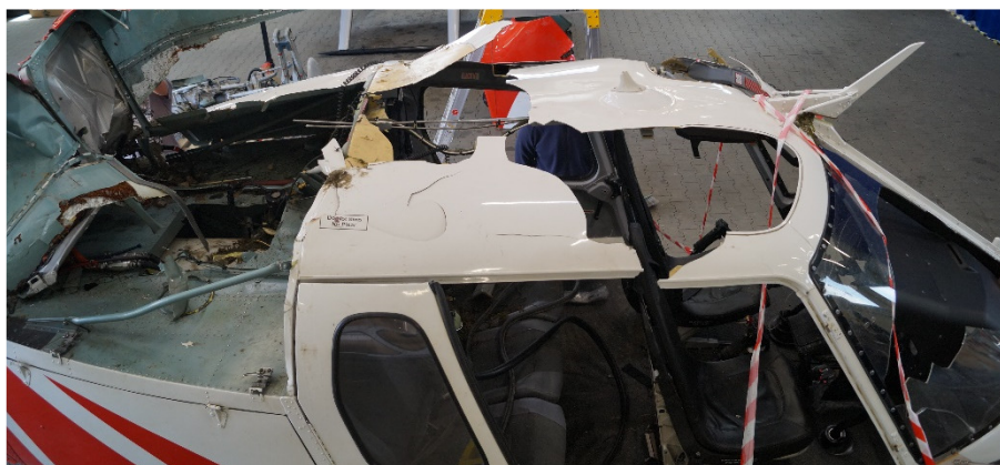
Fig. 3 The wreck after recovery, during an inspection in the Operator's hangar. Visible the area of gearbox mount, cracked skin of the fuselage and broken windshield [source: SCAA]
