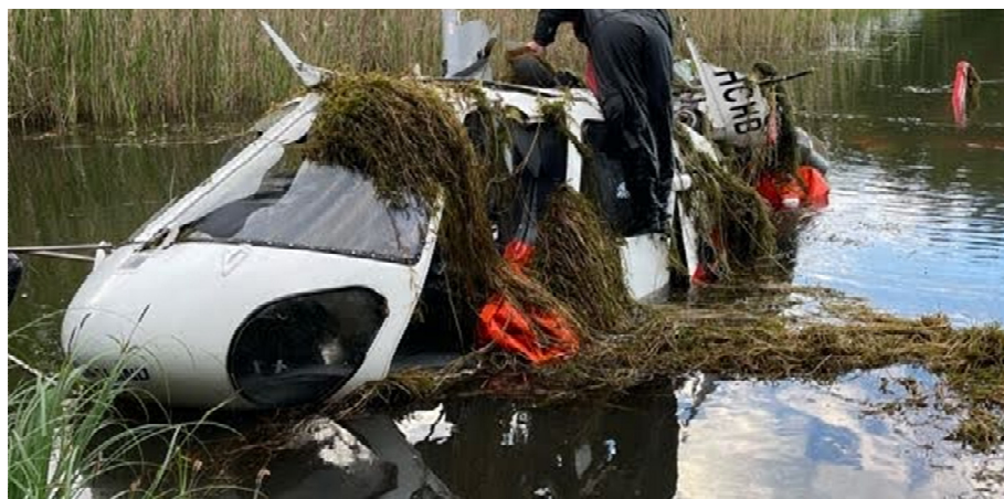
Fig. 2 Helicopter wreckage during recovering to the lake shore. The main rotor and its gearbox were recovered separately [source: SCAA]
