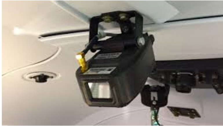
Fig. 8 The APPAREO Vision 1000 camera [source: helicopter manufacturer]
