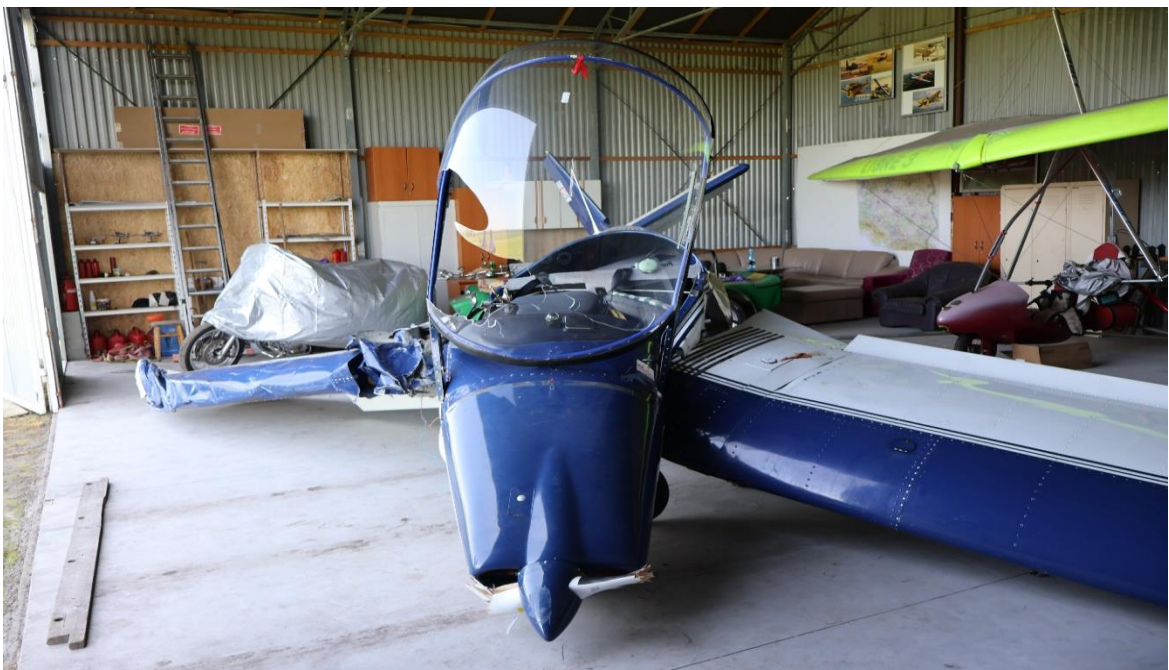
Figure 4. The view of the damage to the propeller and left wing of the aeroplane.
