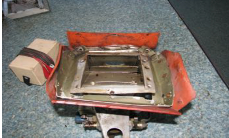
Fig. 11. A view of the hot air throttle with a deformed air intake housing.
