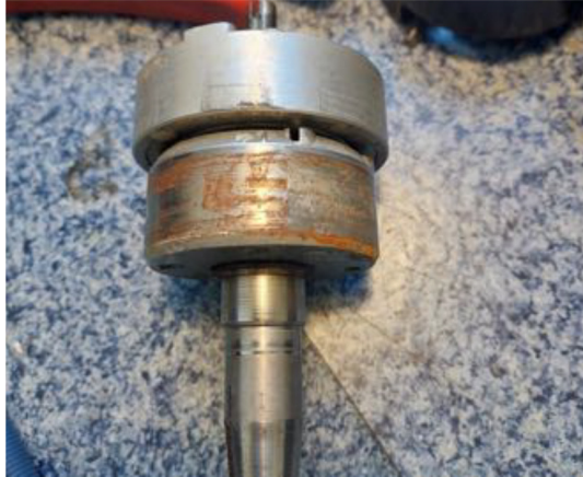
Fig. 9. Corrosion visible on the magneto's stator.
