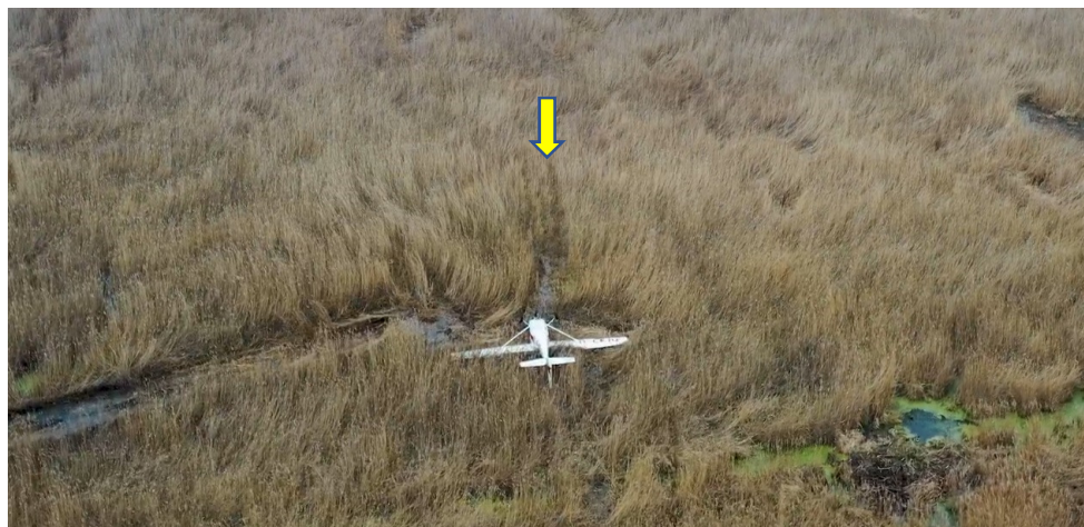
Fig. 2. The position of the airplane after overturn, with the touchdown point marked by a yellow arrow
