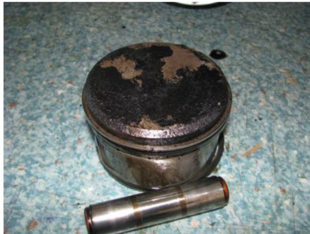
Fig. 12. A dark carbon deposit visible on a piston.
