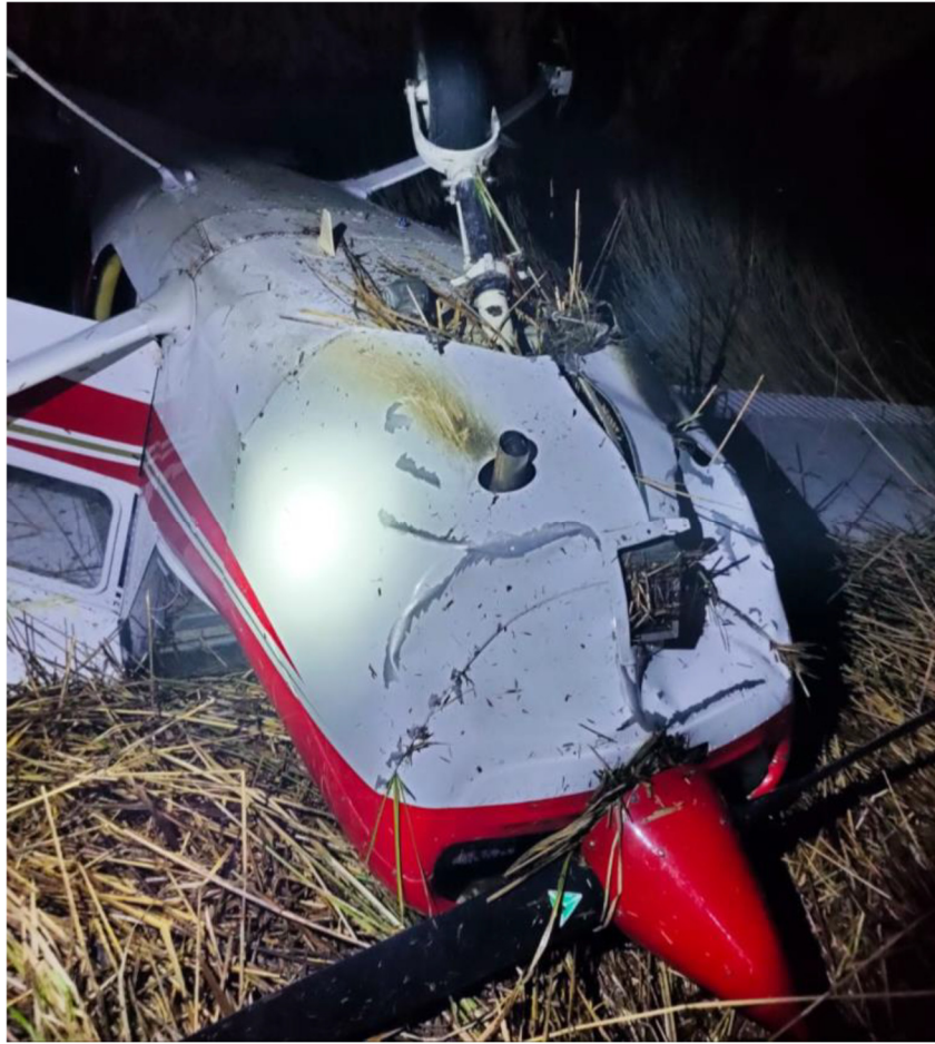
Fig. 6. A view of the damage to the nose section of the fuselage.
