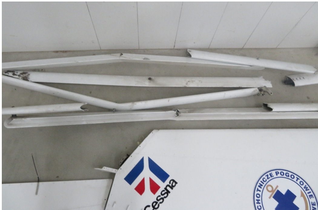
Fig. 2. Broken and bent float struts
