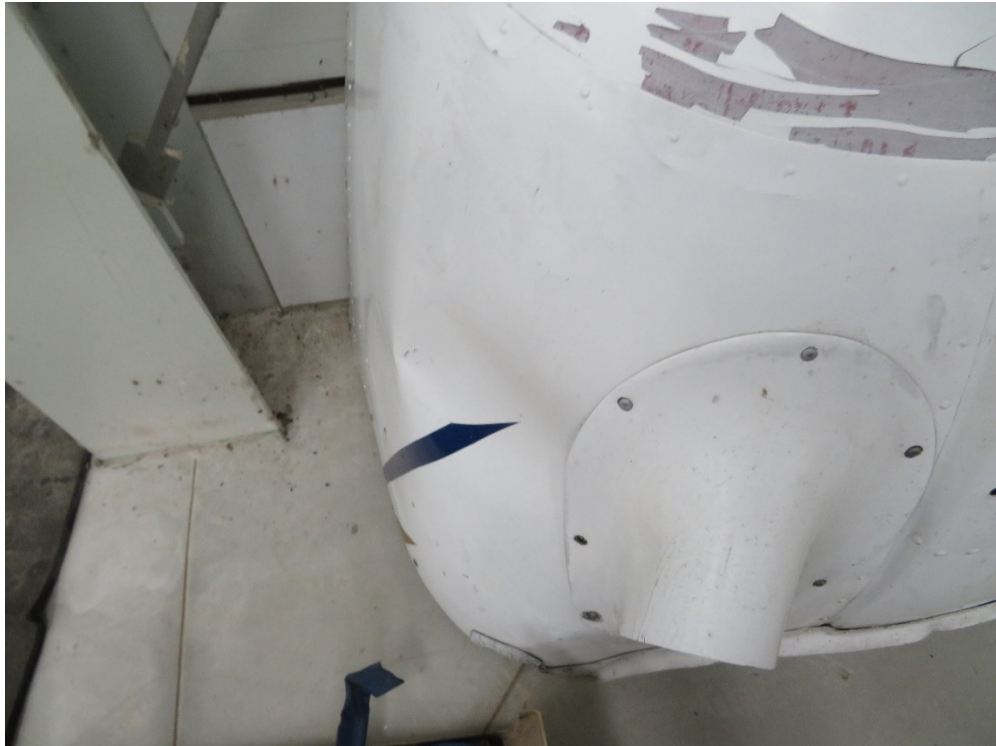
Fig. 3. Dents in the lower engine cowling
