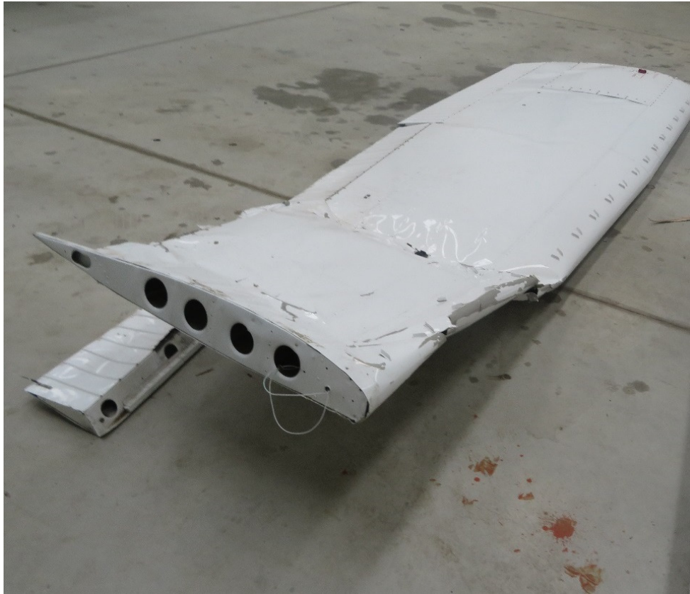
Fig.1. Destroyed right wing with the broken-off aileron
