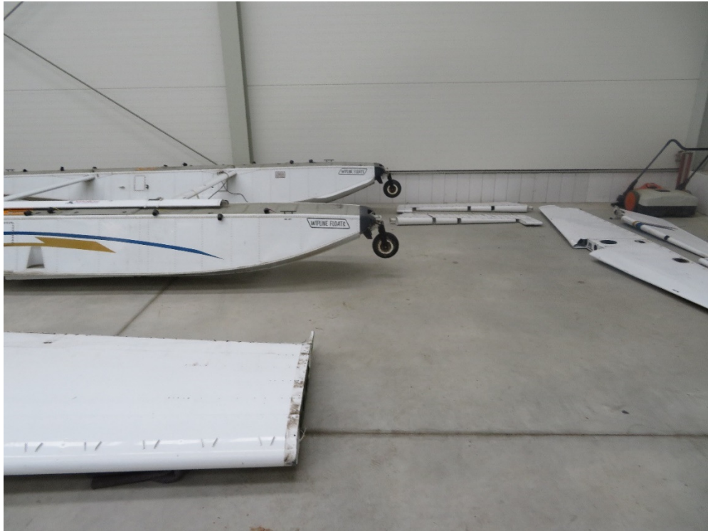
Fig. 5. Deformed and dislocated float mounting elements
