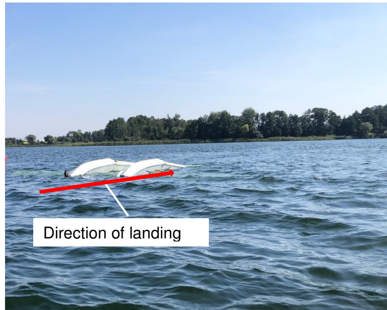
Fig. 8. The aeroplane after overturning, with the deviation to the left visible.
