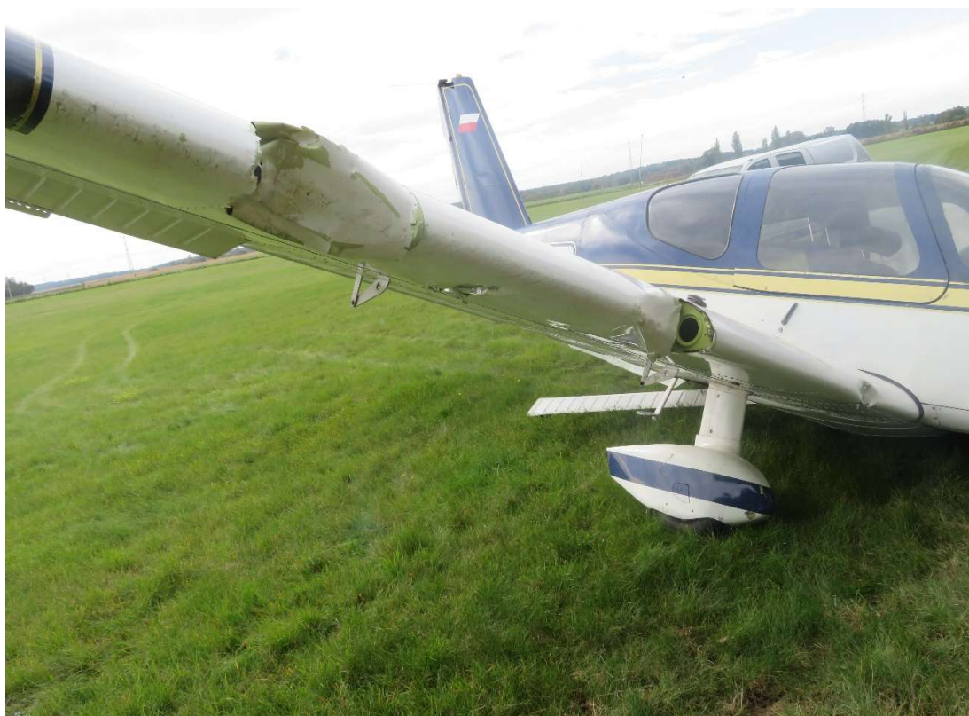
Fig. 3 Damage to the leading edge of the right wing.
