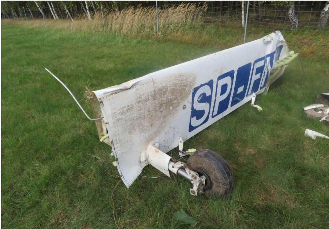
Fig. 4 The separated left wing.
