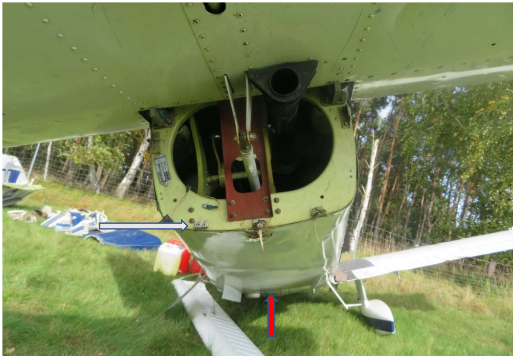
Fig. 5 Damage to the tail section of the fuselage (the fairing missing and dents in the lower fuselage) [source: PKBWL]
