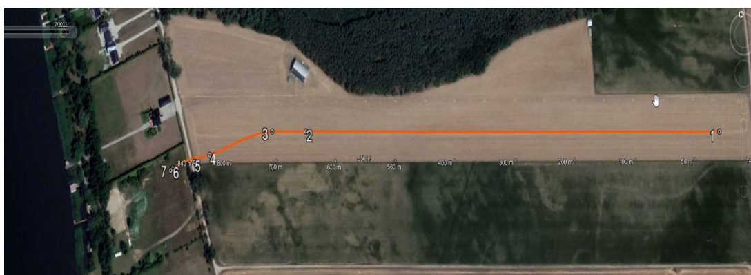
Fig. 8 The aeroplane's take-off route: 1 - the start of the take-off run; 2 - lift-off and flight with critical angles of attack (650 m); 3 - turn to the left; 4 - the tail hits the ground; 5 - the collision with the fence; 6 - the place where the left wing came off; 7 - the place where the aeroplane came to a stop [source: PKBWL]
