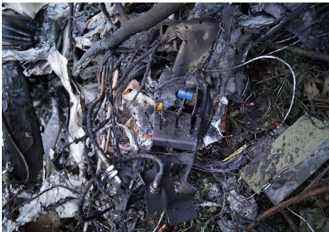
Fig. 10 Engine control system elements found at the occurrence site
