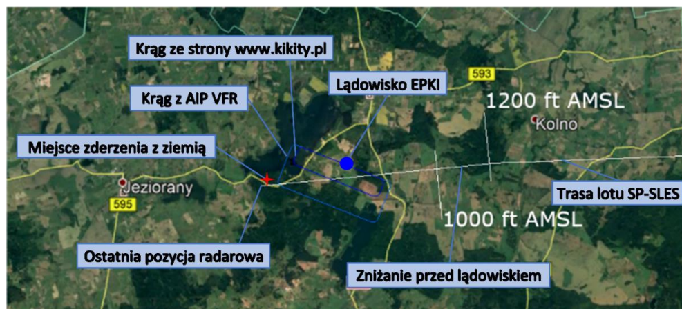
Fig. 1 Final portion of the flight path based on a radar screenshot [source: PKBWL 1 ]
