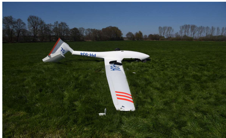
▲ The glider after the ground loop. (Source: Dutch Aviation Police)
